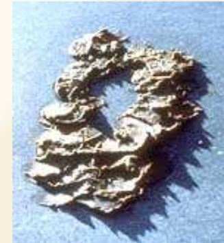
Graffiti removed from historic building with poultice
